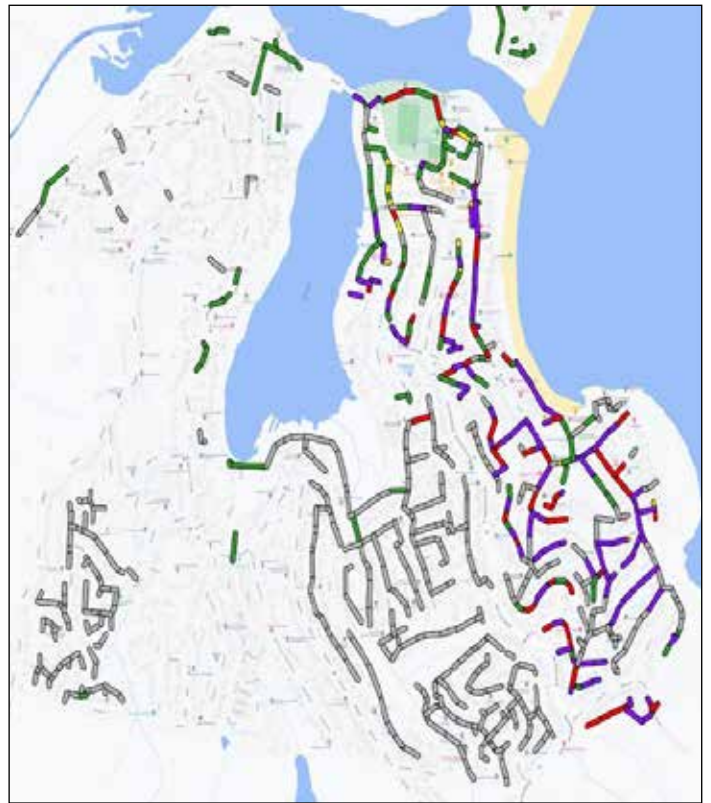
Progress on assessing condition of sewer pipes. Bright colours show lengths investigated so far and ranking of their condition. Red and purple sections will be relined by mid-2023. Grey sections form part of current phase but still to be inspected.
