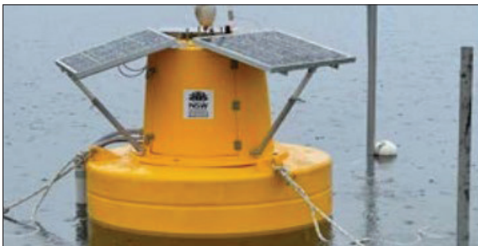
Figure 1: Beatrice an innovative water quality logger
